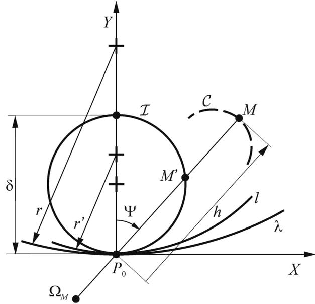
Fig. 3 Inflection circle and cubic of stationary curvature
