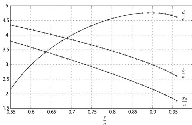
Fig. 17 Design chart for slider-crank mechanisms with quasi-constant transmission ratio
