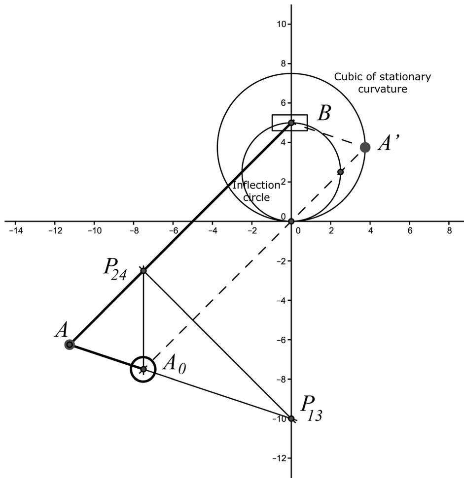
**Fig. 9 Burmester theory: slider-crank mechanism**
