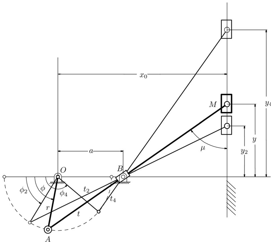
Fig. 11 Chebyshev theory: slider-crank mechanism
