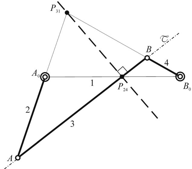
Fig. 1 Freudenstein theorem: four-bar linkage
