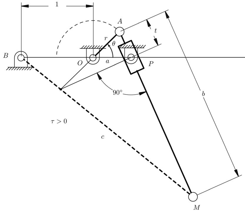
Fig. 12 Chebyshev theory: four-bar linkage for  $\tau > 0$ ,  $a < 1$ , and  $t_0 > 0$
