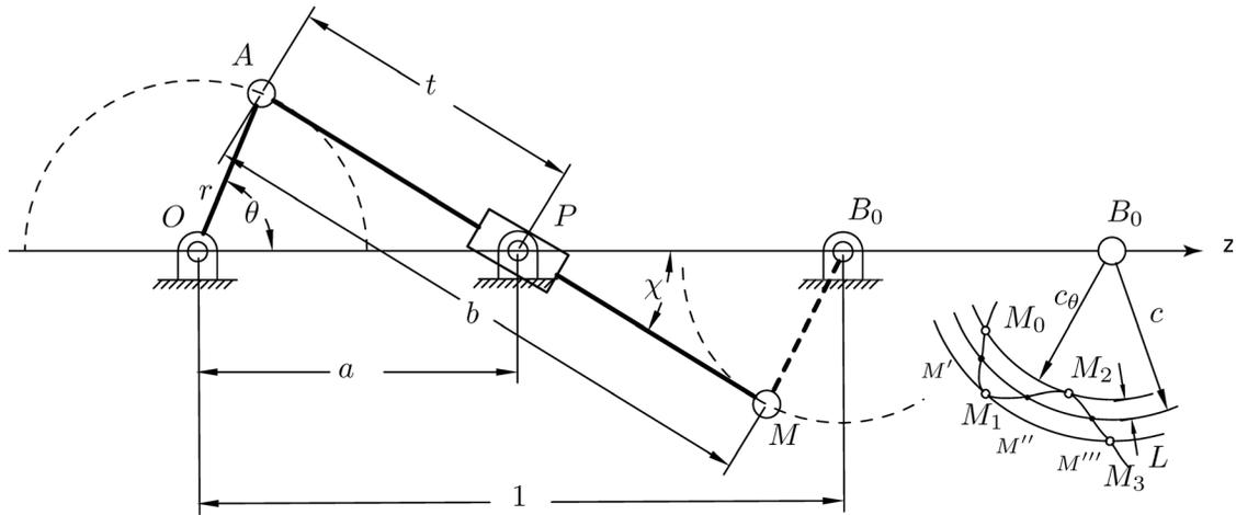
Fig. 10 Swinging-block circular path generator
