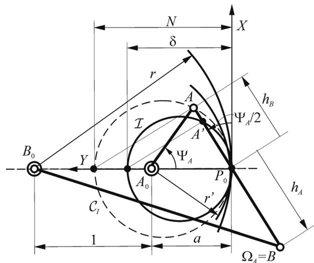
Fig. 4 Burmester theory: four-bar linkage
