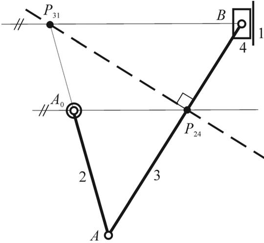
Fig. 2 Freudenstein theorem: slider-crank mechanism
