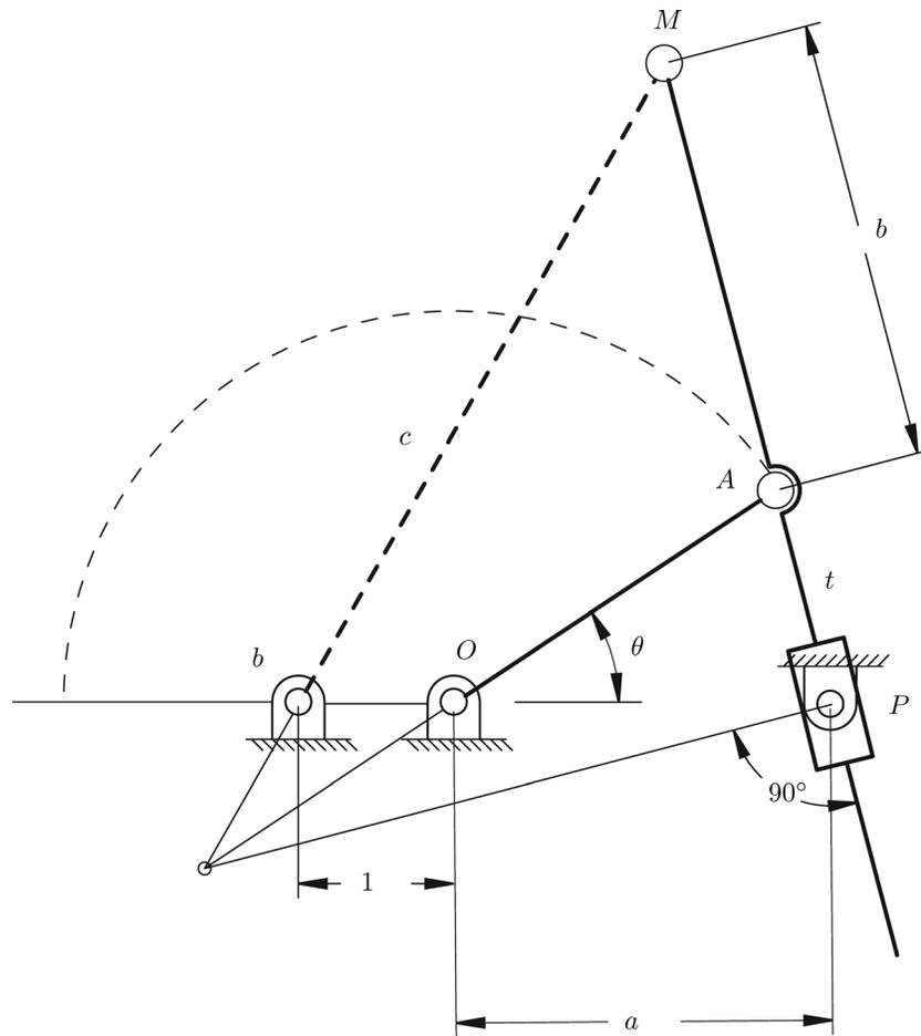
Fig. 13 Chebyshev theory: four-bar linkage for  $\tau > 0$ ,  $a > 1$ , and  $t_0 < 0$
