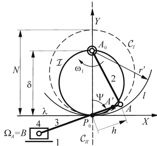
Fig. 7 Burmester theory: slider-crank mechanism
