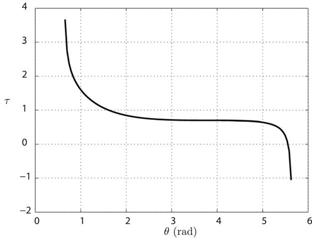
Fig. 14 Four-bar linkage: quasi-constant transmission ratio
