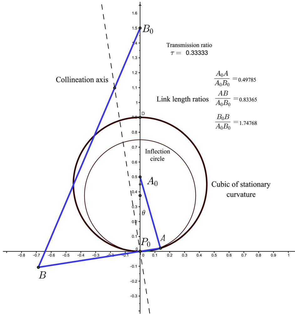
Fig. 5 Burmester theory: four-bar linkage
