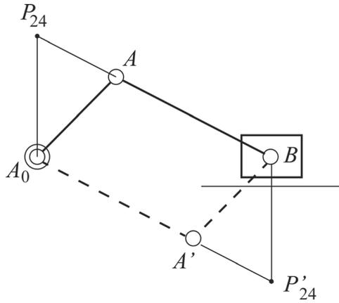
**Fig. 8 Slider-crank mechanism (continuous-line) and its auxiliary mechanism (dashed-line)**
