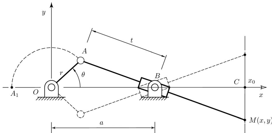
Fig. 15 Swinging-block straight path generator
