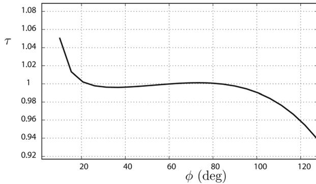
Fig. 16 Slider-crank mechanism: quasi-constant transmission ratio
